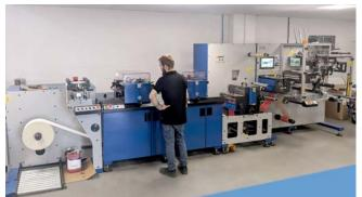
Positive ID Labels' Daco TD350P flexo press with in-line finishing
