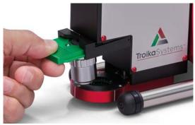
New Kinematic Quick-release lens fitting system guarantees accurate lens placing time after time.
