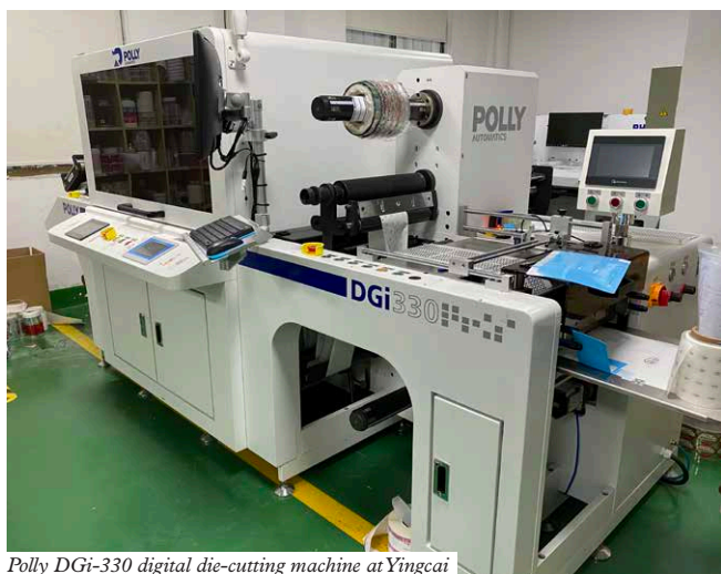
Polly DGi-330 digital die-cutting machine at Yingcai
