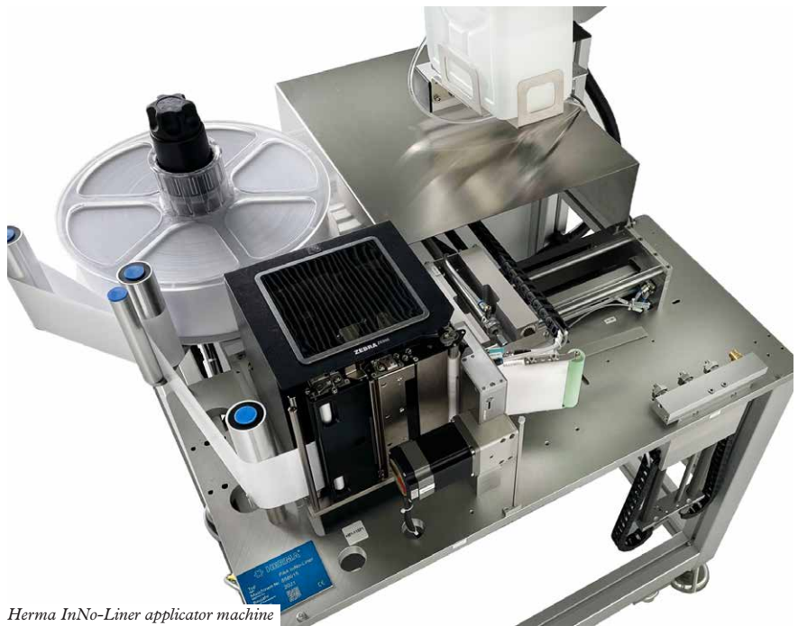
Herma InNo-Liner applicator machine
